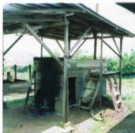
Figure 18. Kiln drying of coconuts requires a clean source of fuel to produce light copra.
