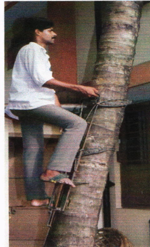
Figure 7. Palm tree climbing device serves as a portable ladder to facilitate tree ascent.
