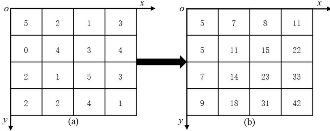
FIGURE 2. The computation of an integral image, (a) A simple image, (b) The integral image
