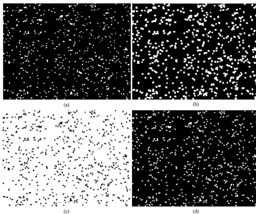
FIGURE 7. Comparison of segmentation results, (a) Global threshold method, (b) Intra-class variance threshold method, (c) Iterative threshold method, (d) Method in this paper
