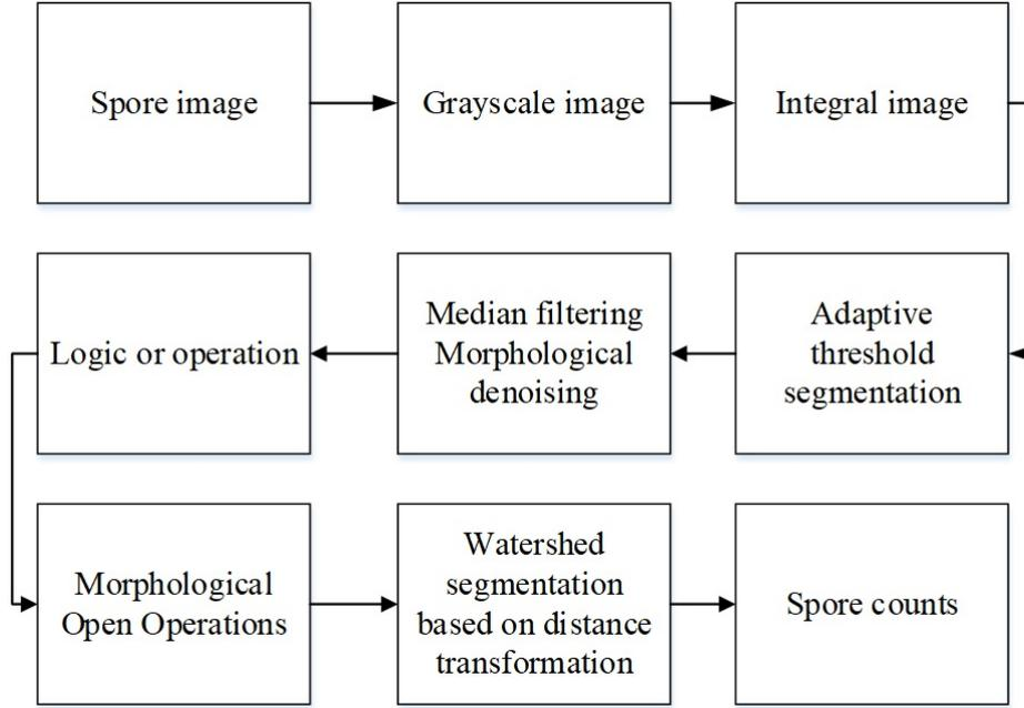
FIGURE 1. Flow chart of spore counts method
