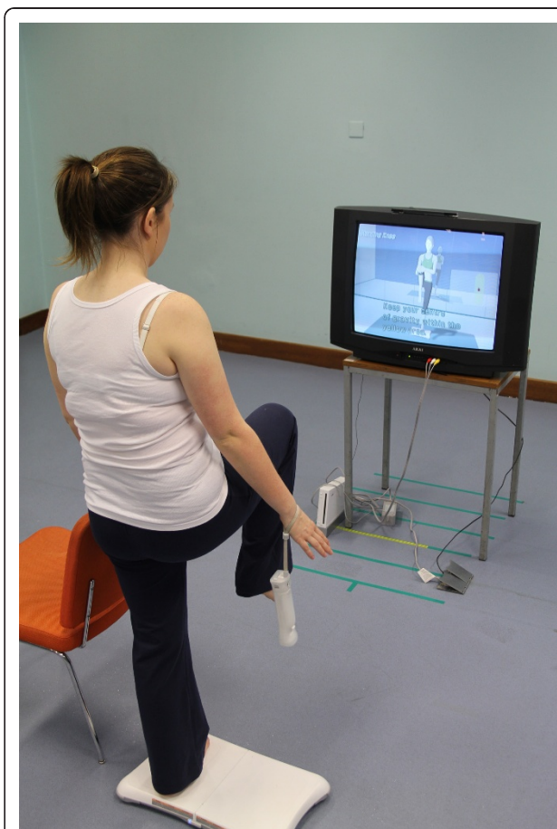
Figure 1 The Nintendo Wii Fit Plus®. The participant stands on the Wii balance board which monitors centre of pressure and reconstructs it visually on the television monitor as a red dot within a yellow area. A variety of exercises and games are available to retrain balance and encourage head movement. Stepping exercises can also be performed encouraging stopping and changing direction, in which the vestibular system has a role. Written consent to reproduce the image was provided by the subject in the photo.
