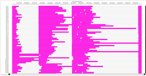
Fig. 2. LP solves, which are the smallest unit of computation, display sizeable variation in time to solution. This variation is not predictable too. Hence, the blocks of sequential computation do not display any persistent performance behavior that can be exploited. This plot shows a sample execution profile (on several processors) of evaluating multiple Stg2 scenarios for candidate Stg1 solutions. Colored bars represent an LP solve, while white stretches are idle times on that processor. Each processor (horizontal line) is assigned a specific Stg2 scenario, and evaluates multiple candidate solutions from Stg1 one after the other. Some loose synchronization is introduced so that every vertical grouping of bars represent the times taken for the evaluation of different scenarios for the same candidate solution from Stg1. We observe a wide variation and no persistence, both across scenarios and across candidate solutions. This illustrates the shortcomings of a static decomposition of the available work across processors.
