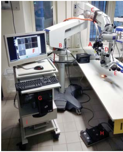
Fig. 2: Overview of the spectral video camera in the clinical environment. (A) Seven-band spectral video camera, (B) Zeiss OPMI Vario S88 surgical microscope, (C) lifting arm of the suspension system with attached spectral video cabling, (D) main binocular tube for the lead surgeon, (E) the flexible foldable tubular for a surgeon's assistant, (F) screen with the customized software and the real-time preview from spectral video camera, (G) computer with a dedicated frame grabber, (I) multi-Purpose medical cart with electrical transformer, (H) foot control panel allowing to control different surgical microscope functions.
