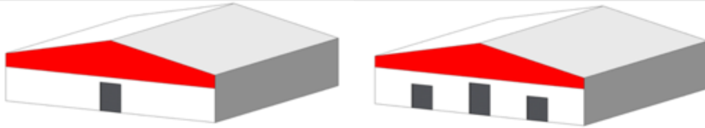
Figure 68 Permitted signboards for closed storage and warehouses
