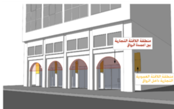
Figure 62 Position of signboards within arches
