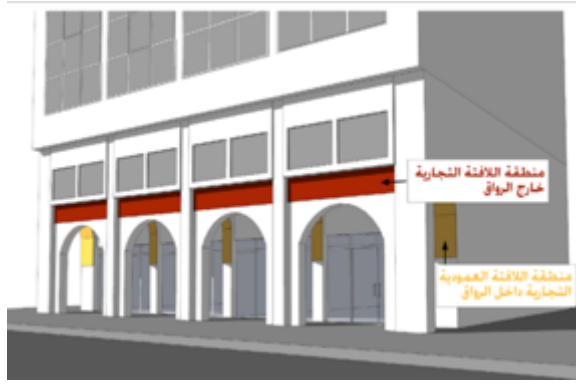
Figure 64 Permitted location of ground floor signboards on passage exterior and interior
