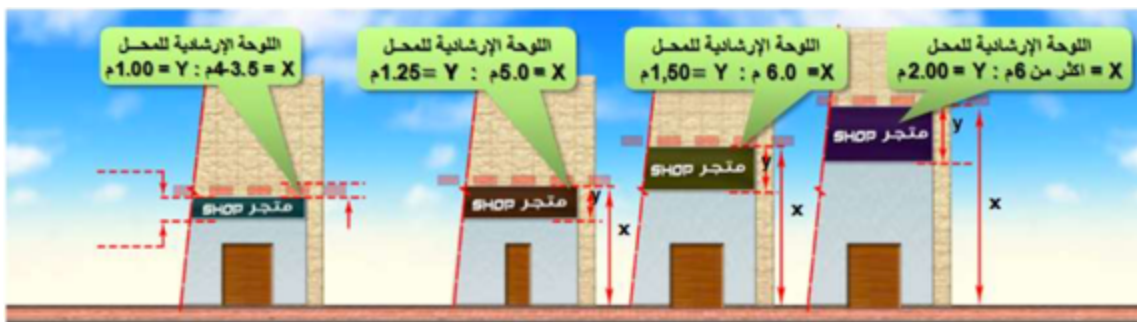
Figure 81 signboard placement depending on building design and height
