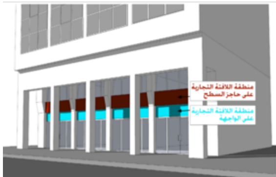
Figure 61 Position of signboard within covered passages
