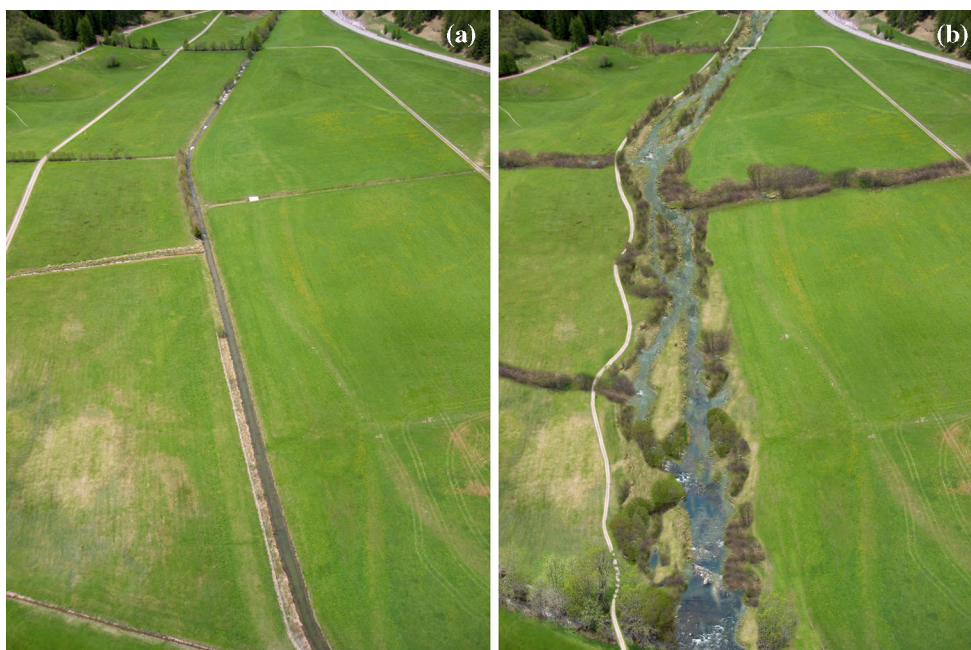
Fig. 7 Rombach at Fuldera a before restoration and b an animation of the planned outcome after restoration of the Rombach (© Pio Pitsch)
