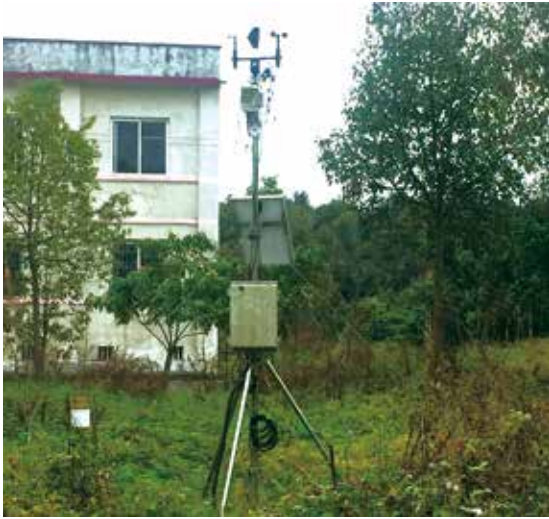
Automatic meteorological observation station
