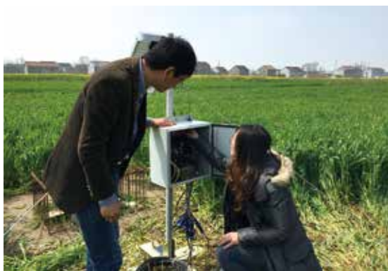
Checking the automatic monitoring equipment for soil water-salt dynamics
