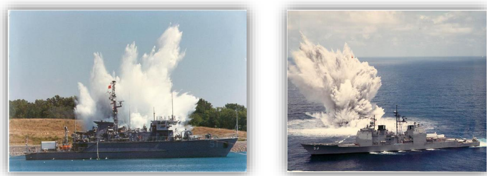
Figure 1. 9 USS OSPREY-MHC 51(left) [9] and CG 53(right-Courtesy of U.S Navy) Ships Full-Scale Shock Trials
