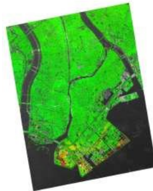
PALSAR-1 PSI example over Chiba, Japan. The average deformation rate is shown using a color scale between -2.5cm/year (red) and +2.5cm/year (blue).
