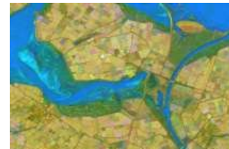
RGB composite of ERS coherence (red), average backscatter (green), and backscatter temporal variability (blue) over the Netherlands.
