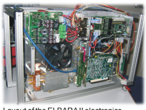
Layout of the ELBARA II electronics.
