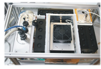
Layout of the ELBARA II electronics.
