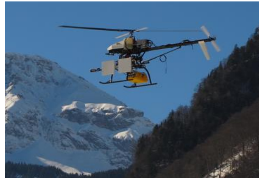
GAMMA L-band SAR on Aeroscout's VTOL UAV Scout B1-100, equipped with a Honeywell HGuide n580 INS/GNSS navigation system, at the test site Wolfenschiessen, Switzerland.
