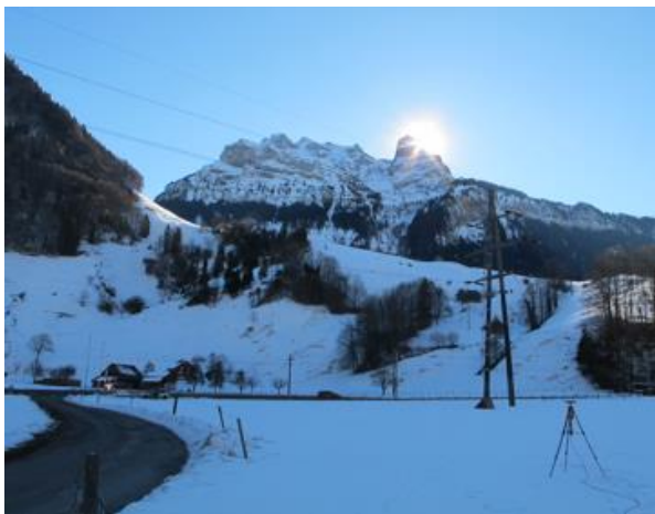
Area of interest on the campaign day. On the lower right, the local GNSS reference station is situated to obtain a highly precise post-processed kinematic GNSS solution of the UAV position.
