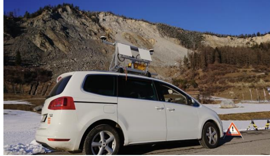
Car-borne Gamma L-band SAR setup with Honeywell HGuide n580 INS/GNSS system at the Brinzauls landslide.
