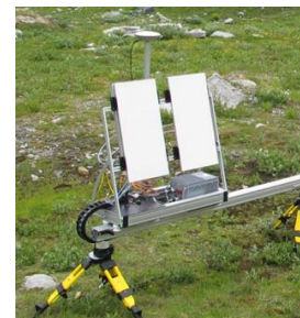
Rail-based terrestrial measurement setup with the GAMMA L-band SAR to autonomously acquire short interval time series of repeat-pass interferometric SAR data of a glacier.
