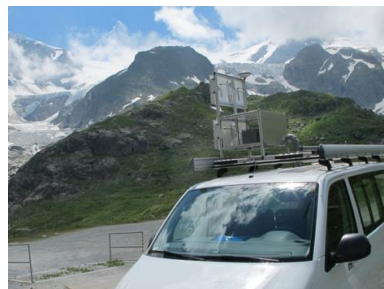
GAMMA L-band SAR mounted on a car during a demonstration campaign in cooperation with ETH Zurich. A ring-laser-gyro INS/GNSS system (iNAV-RQH) by iMAR Navigation GmbH was used for high-precision positioning and attitude determination. GNSS data is processed in post-processing kinematic mode with an ad-hoc local GNSS reference station in the field. SAR antenna/channel configuration: on transmit/ three receive antennas.
