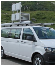
Car-borne setup of the L-band SAR system with one transmit and three receive antennas. Repeated SAR data acquisitions of the Stein Glacier were made while driving on a slightly curved section of mountain road.
