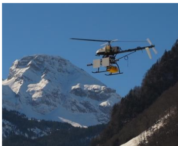
The GAMMA L-band SAR mounted on Aeroscout's UAV Scout B1-100 during an interferometric repeat-pass SAR data acquisition in Switzerland. The UAV is equipped with a Honeywell HGUIDE n580 INS/GNSS system. GNSS data is processed in post-processing kinematic mode with an ad-hoc local GNSS reference station in the field. SAR antenna/channel configuration: one transmit/ one receive antenna.
