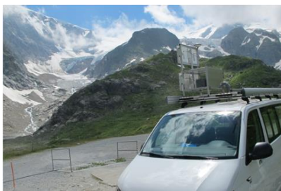
Car-borne setup of the L-band SAR system with one transmit and three receive antennas. Repeated SAR data acquisitions of the Stein Glacier were made while driving on a slightly curved section of mountain road.
