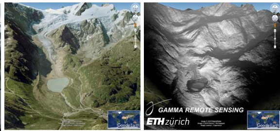
Google Earth view (left) of the Stein Glacier test site (CH). Geocoded intensity image (right) overlaid to Google Earth view as obtained from a car-borne L-band SAR acquisition.
