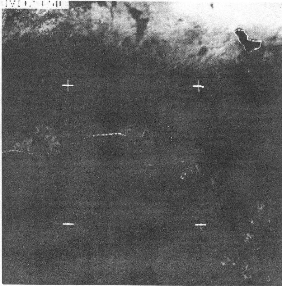
Fig. 2. Map of the reference albedo of western Central Africa, obtained from Meteosat data received in WEFAX format for the last days of January 1984. The albedo increases from black to white.
