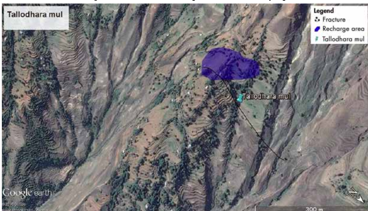
Figure 7: Demarcation of recharge area for Tallodhara spring
