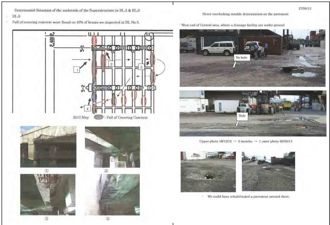
Figure 1.5-3 Results of Inspection Performed in 2013
