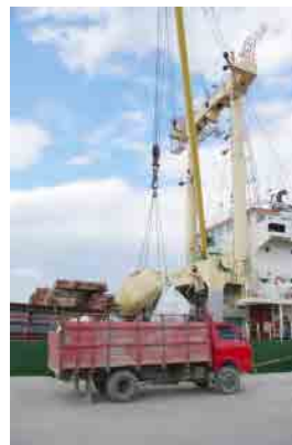
Figure 6.1-2 Quay-side Handling of Bag Cargo (cement)
