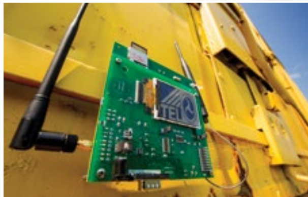
Sensor mounted on railcar
