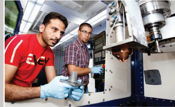
Graduate research assistants Haitham Hadidi and Cody Kanger use the Optomec Lens 3D Hybrid Machine.
