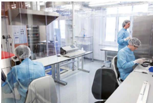
HuCE has setup and runs a certified clean room class 8, used for medical device manufacturing in the building of Innocampus/Switzerland Innovation Park, Biel.
