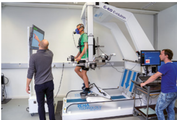
G-EO end-effector gait rehabilitation robot augmented at IRPT with biofeedback for cardiopulmonary testing and training.
