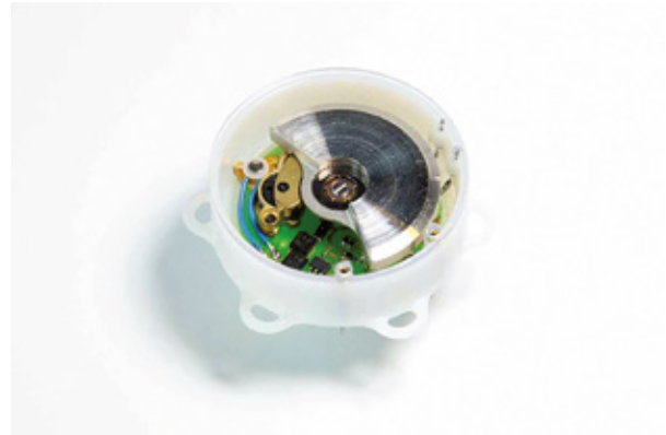
Prototype of a lead- and batteryless cardiac pacemaker (courtesy of the Group for Translational Electrophysiology, Department of Cardiology, Bern University Hospital & ARTORG Center for Biomedical Engineering Research).
