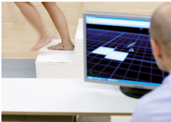
Set of four markers to measure the navicular bone kinematics under dynamic loading.
