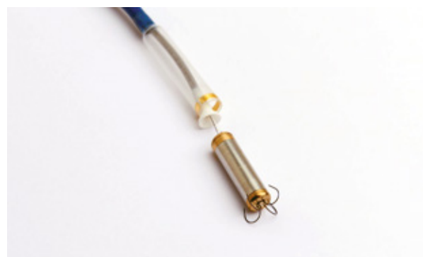
Prototype of a lead- and batteryless cardiac pacemaker.
