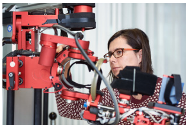
Rehabilitation Robot ARMin for optimized motor learning (R. Riener & T. Nef).
