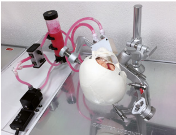
Complete single-patient customized simulation model, consisting of a pressure-adjustable pulsatile pump, rheology fluid a missing words?
