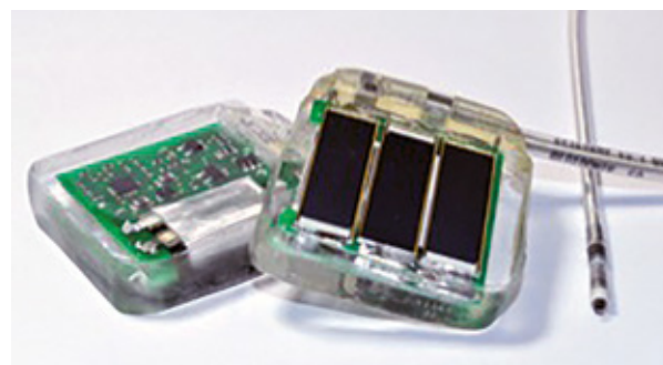
Prototype of a batteryless cardiac pacemaker powered by solar cells.
