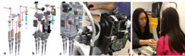
Left: (a) 3D optical arrangement, (b) added compact mounting elements, (c) additive-manufactured uni-body. Right: (d) Integrated measurement head (without cover) and (e) completed user interface during study of myopia progress in children.
