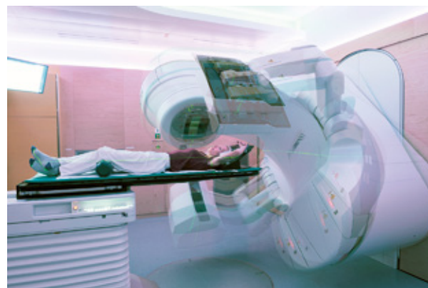
Dynamic trajectory delivery is based on the possibility to move and rotate many delivery components simultaneously.
