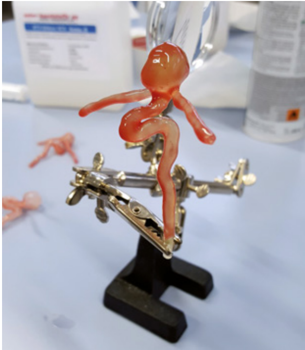
Ultra-thin silicon layered, single-patient customized aneurysm model
