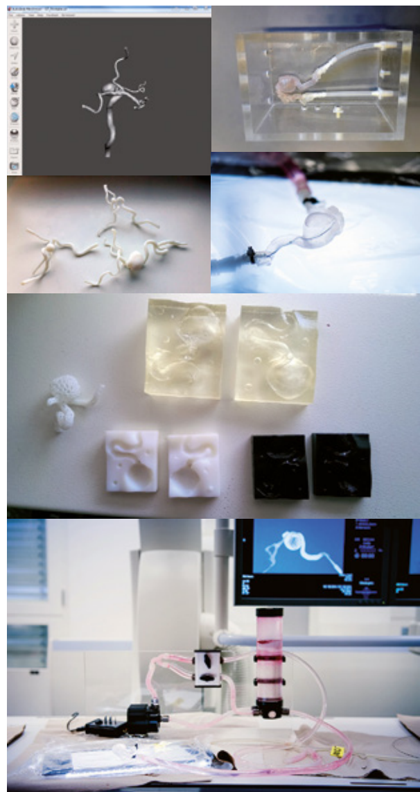
Developmental process of cerebral aneurysm models using additive manufacturing techniques (3D printing) based on patient specific 3D imaging data sets.
