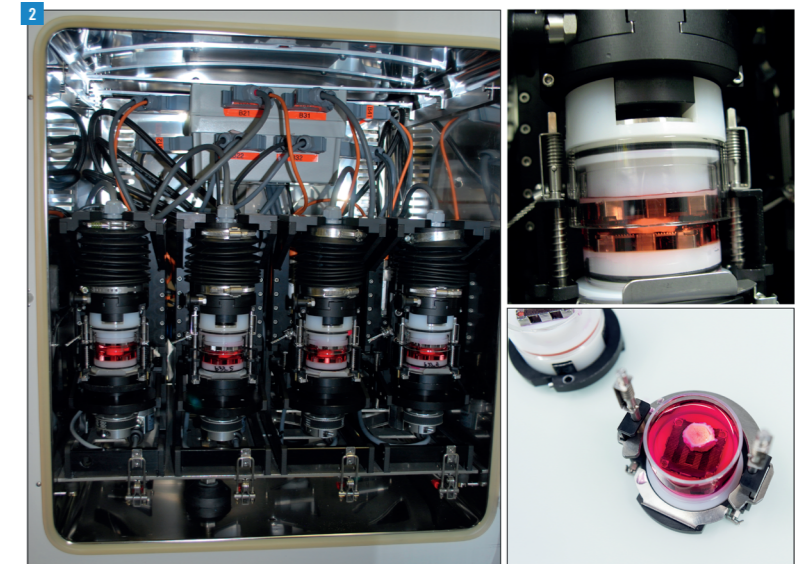
Specialized Bioreactor to apply compression and torsion for culturing entire units of bovine-derived intervertebral disc explants in organ culture under compression and torsion. Left: inside incubator, upper right: close-up view of culture chamber, lower right: inside view of culture chamber with positioned bovine coccygeal intervertebral disc. This device is worldwide unique.
