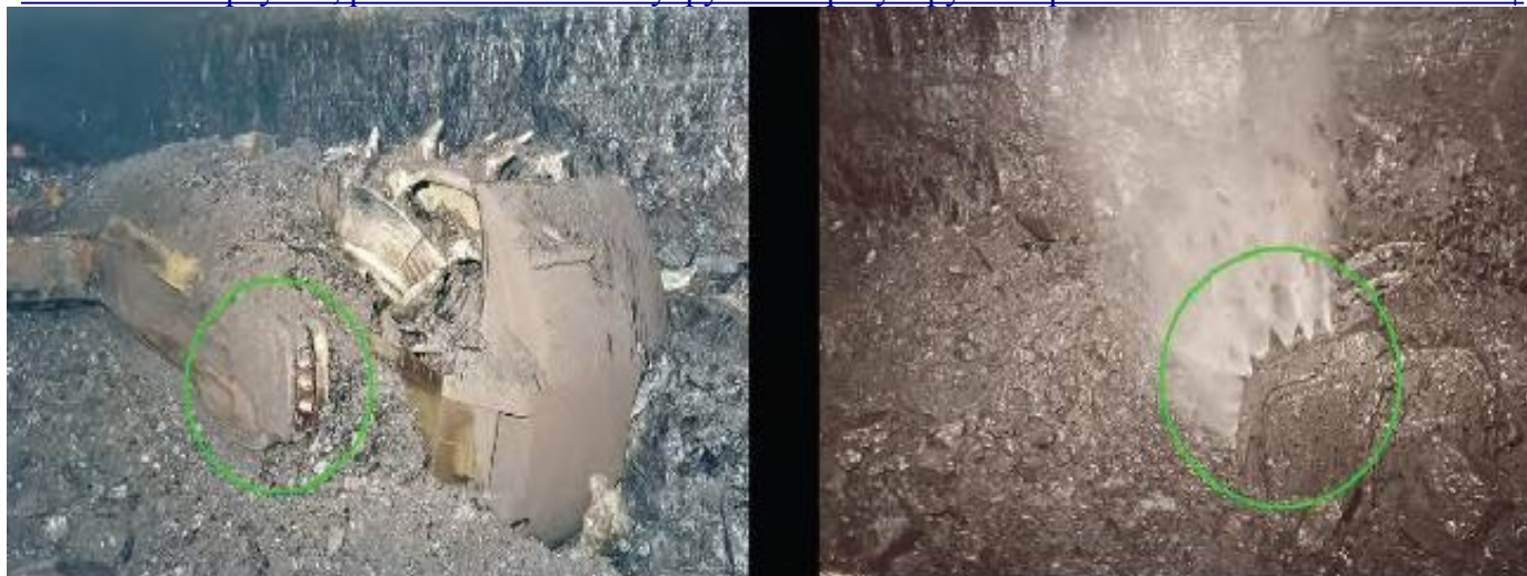
Figure 3-13.—Crescent sprays located on shearer ranging arm.
