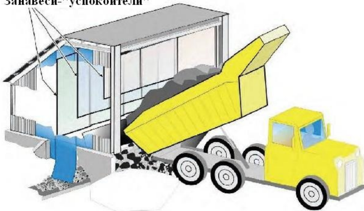
Figure 5-4.—Staging curtains used to prevent dust from billowing out of enclosure.
