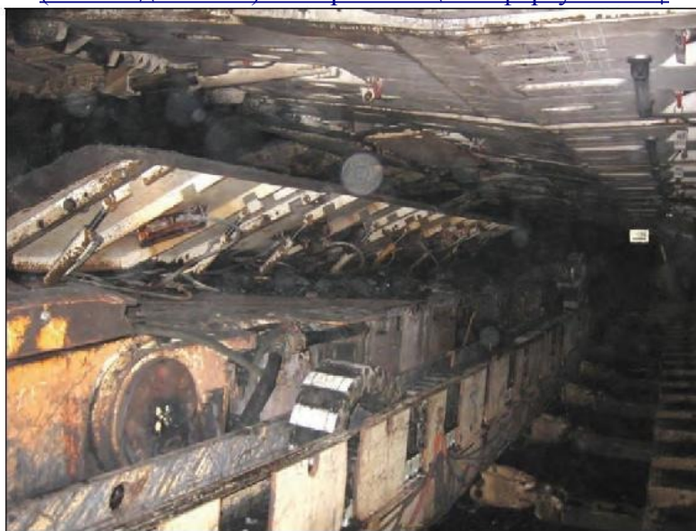
Figure 3-12.—Raised deflector plate can enhance the effectiveness of the directional spray system.
