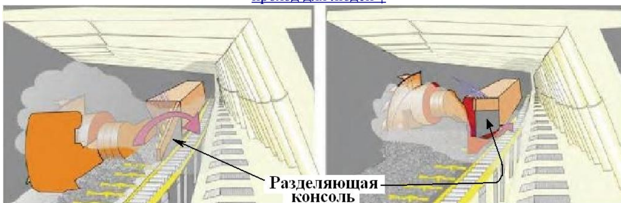
Figure 3-11.—Position of splitter arm may allow dust to migrate into walkway.
