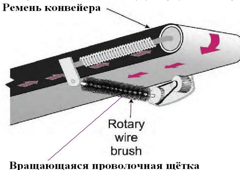
Figure 3-1.—Rotary brush cleans the conveying side of the belt.
