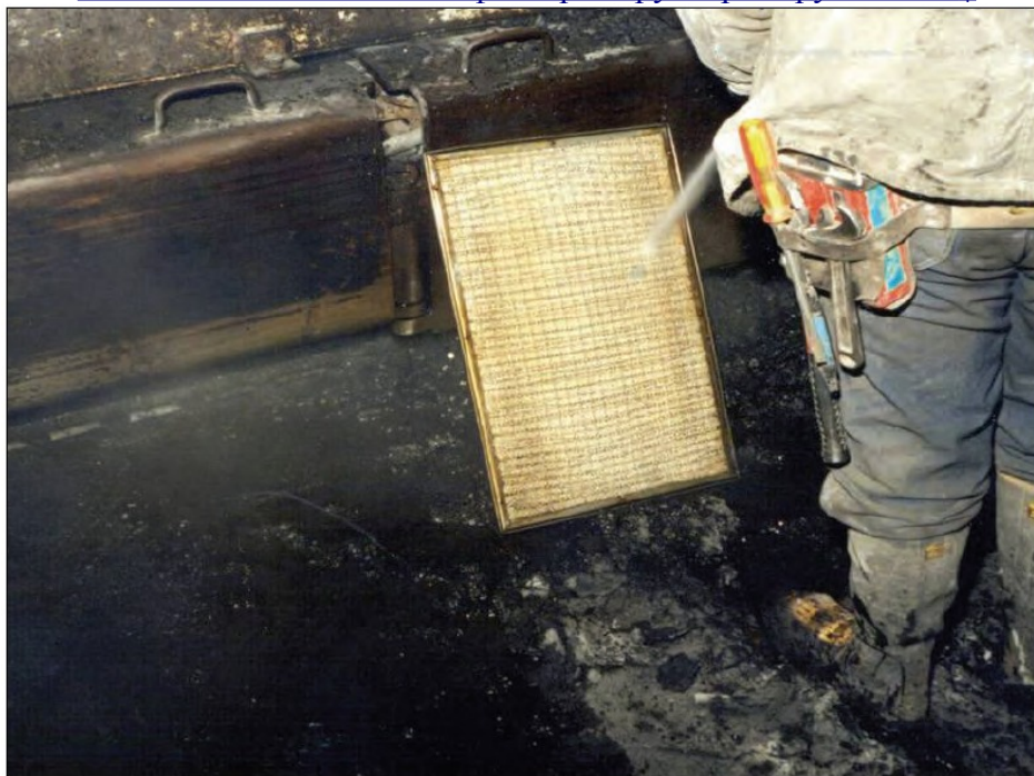
Figure 4-7.—Cleaning scrubber filter panel with water spray.
