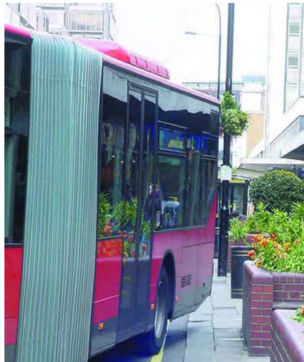
Rear section of bus overhanging footway as it exits stop
