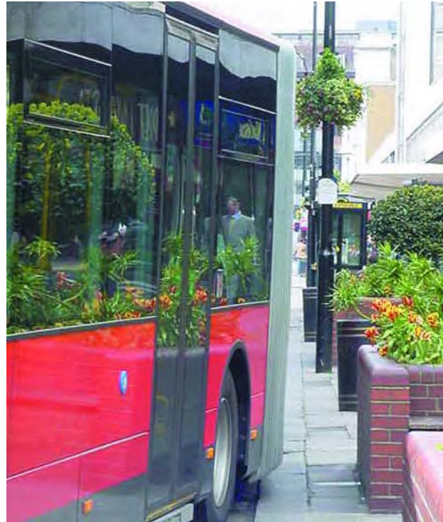
Centre section of bus overhanging footway as it exits stop
