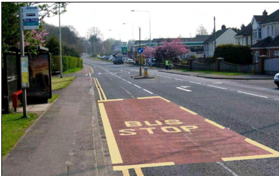
Photo 8f – Typical NI carriageway markings
