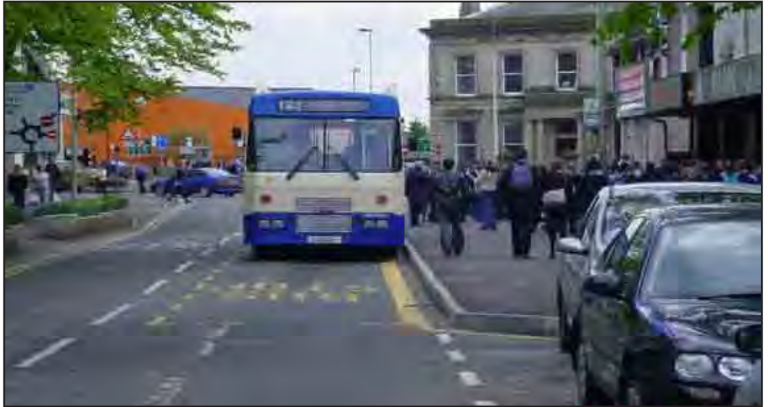
Photo 7i – Full width bus boarder
