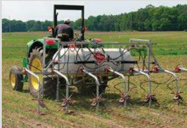
Photo 11.1. Flame weeder with torches directing flames on both sides of the crop. The height, direction, and angle of the torches are adjustable (Photo credit: Michigan State Univ. Extension Bulletin E-3038).
