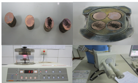
Fig. 1. Foto proses coating sampel JEO. L JFC-1600 Auto Finen Coater and SEM-EDS JEOL JESM 6510 LA
