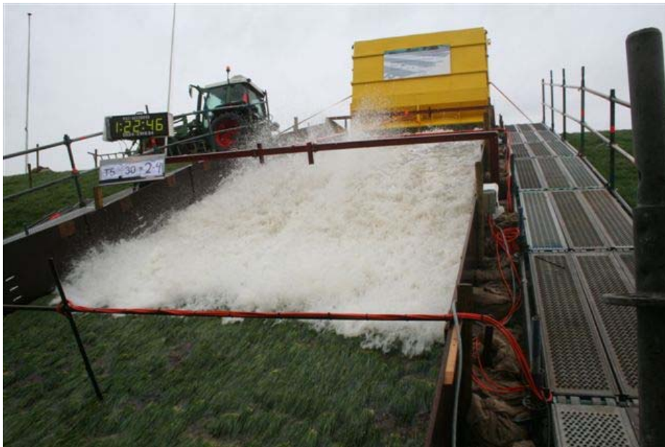
Figure 3.5: The wave overtopping simulator discharging a large overtopping volume on the inner slope of a dike
