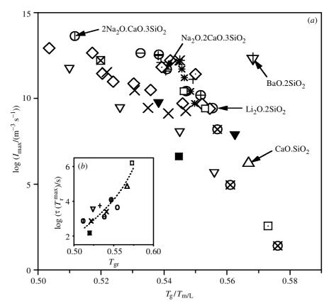
Figure 1. (a) Maximum nucleation rates against  $T_{\rm gr}$  for 51 glasses of stoichiometric compositions and non-stoichiometric compositions. (b) Time-lag of nucleation at  $T_{\rm max}$ . (After Fokin et al. (2002a).)
