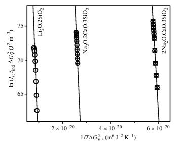
Figure 3. Plots of  $\ln(I_{\rm st}t_{\rm ind}\Delta G_{\rm v}^2)$  against  $1/T\Delta G_{\rm v}^2$  for three stoichiometric glasses. Linear fit for  $T>T_{\rm g}$ .  $\Delta G_{\rm v}$  corresponds to  $\Delta C_p=f(T)$ .
