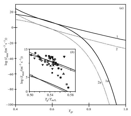
Figure 2. Maximum nucleation rate as a function of reduced glass-transition temperature. (a) The lines are calculated from the CNT with  $T_{0r}=0.4$  (1, 2) and  $C_2=4.5$  (1a, 2a) for different thermodynamic barriers:  $C_1=5$  (1, 1a),  $C_1=7$  (2, 2a). (b) Points refer to experimental data. The lines are calculated from the CNT with  $C_1=4.5$  (1),  $C_1=6.5$  (2). Solid lines,  $C_2=4.5$  and  $T_{0r}=T_{\rm gr}-C_2/30$ ; dashed lines,  $T_{0r}=0.4$ . (After Fokin et al. (2002a).)
