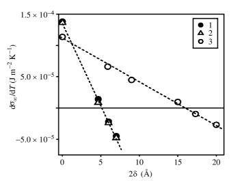
Figure 6. Average values of  $d\sigma_{\infty}/dT$  against Tolman's parameter for Li<sub>2</sub>O.2SiO<sub>2</sub> (1, 2) and Na<sub>2</sub>O.2CaO.3SiO<sub>2</sub> (3) crystals in parent glasses having the same compositions. The kinetic barrier for nucleation was estimated from time lag of nucleation (2, 3) and viscosity (1). (Reproduced with permission from Fokin & Zanotto (2000).)
