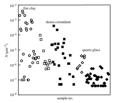
Figure 8. Nucleation density of  $\mu$ -cordierite at cordierite glass surfaces, fractured and annealed under different conditions. O denotes fire-clay furnace, air;  $\square$ , corundum tube furnace, air;  $\triangleleft$ , corundum tube furnace, dust protected;  $\blacksquare$ , corundum tube furnace, dry air;  $\blacklozenge$ , quartz-glass tube furnace, air;  $\diamondsuit$ , quartz-glass tube furnace, vacuum. (Reproduced with permission from Müller (1997).)
