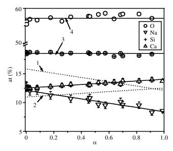
Figure 4. Glass  $1Na_2O.2CaO.3SiO_2$ : compositional variation against volume fraction crystallized at 650 °C. Glass (points) measured by EDS; crystals (dotted lines 1 and 2 denote Na and Ca, respectively) calculated from the parent glass composition and EDS measurements. Solid lines fit the experimental data. Dashed lines 3 (Si) and 4 (O) correspond to the parent glass composition. (After Fokin *et al.* (2002b).)
