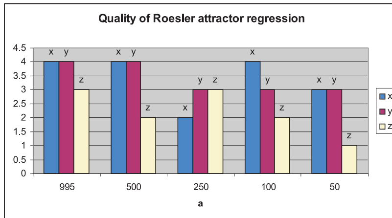
Fig. 6 Average dependency between data set size and quality of result. Magnitudes have the following meaning – 1 is totally different algebraic form of solution, 2 represents decomposed constants and variables, 3 means decomposed constants and 4 is perfect form (equal to generating function).
