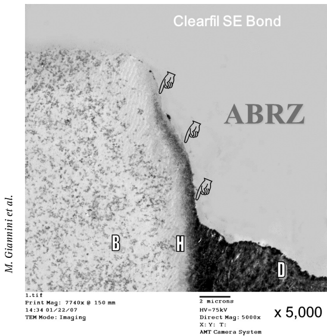
Figure 8. TEM image of the dentin-adhesive interface after acid-base challenge. The TEM/SAED evidence demonstrated that the ABRZ contained densely arranged apatite crystallites (5,000x magnification).
