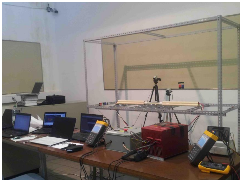
Figure 3. Experiment setup for the measurements. Foreground: reactor control system, the two PCEs for electric power measurements, and one of the multimeters used to verify that no DC components were present. Background: reactor, the two thermal imagery cameras. Note the 6 dosimeters (pairs of red and blue rectangles: 2 on wall, two to the left of reactor, and two to the right, on the far ends of the metal frame) for radiation emission measurements.
