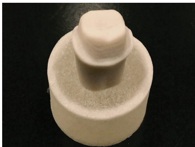
Fig. 1 Prepared ivory tooth (master die).
