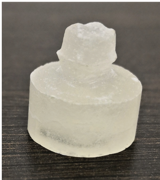
Fig. 2 Duplicated resin die of the master die.
