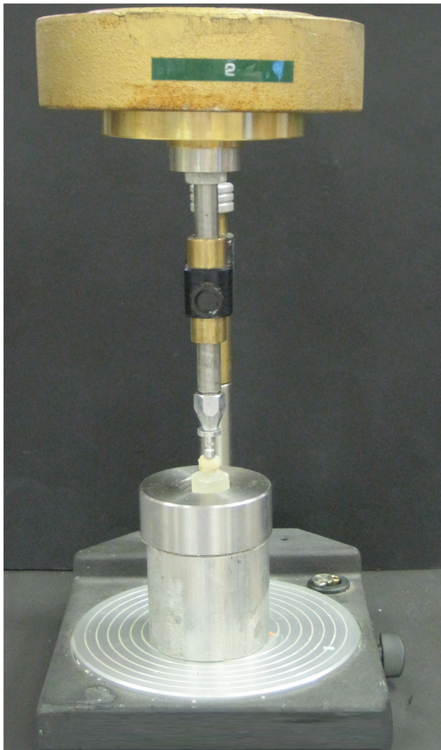
Fig. 4 Customized dental surveyor for standardized loading.
