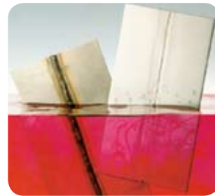
Before and after pickling.
