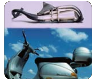
Grade 1.4509/441, Centro Inox, Italy. The new Vespa ET2 is equipped with a ferritic catalytic silencer.
