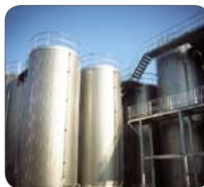
Grade SUS430J1L, coloured-resin coated (outer jacket), JSSA, Japan
