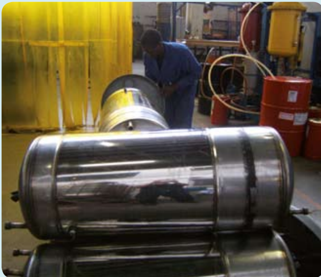
Welded tank, grade 441, S. Africa.
