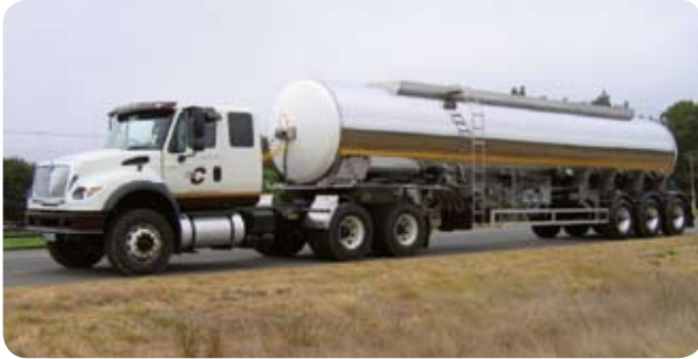
Milk tanker, cladding in grade 430, S. Africa.
