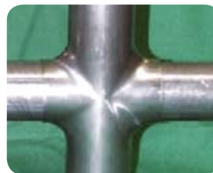
1.4003 hydroformed welded tube.
