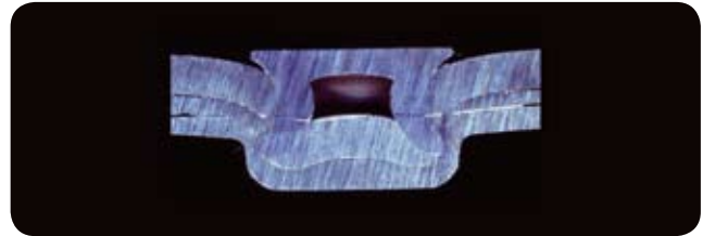
Auto-riveting on 430, 1.5 mm.
