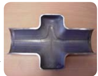
1.4003 hydroformed welded tube.
