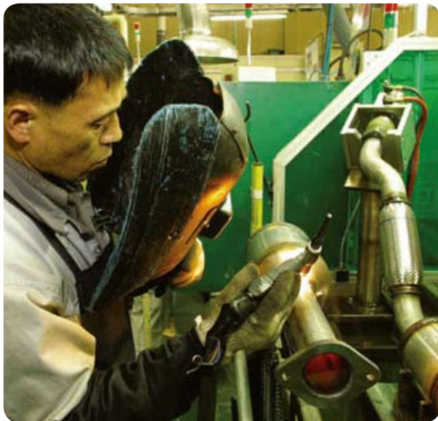
Exhaust system welding, grade 439, S. Korea.
