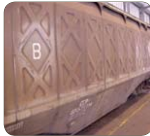
Grade 1.4003/410 (panels), Columbus, S. Africa. In service for over 20 years.
