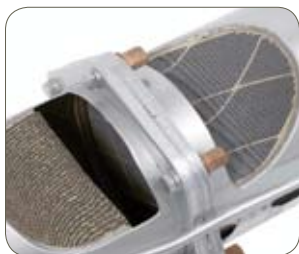
Grade 1.4509/441, diesel particle filter, Peugeot 607, Faurecia
