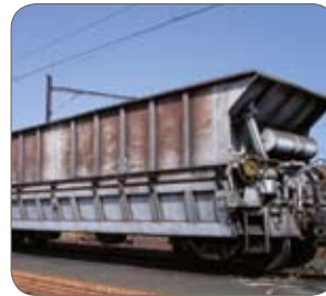
Grade 1.4003/410 (panels), Columbus, S. Africa. In service for over 15 years.
