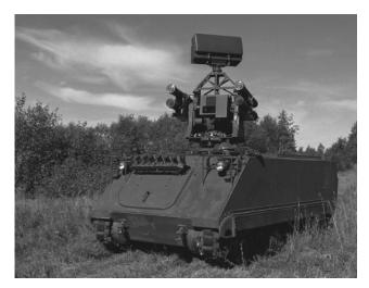
Fig. 6: The ASRAD-R with Bolide missile and the HARD 3D search radar
