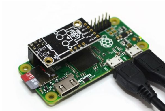
Figure 3.12: An example on how to connect the Raspberry Pi Zero W to the BerryIMU
