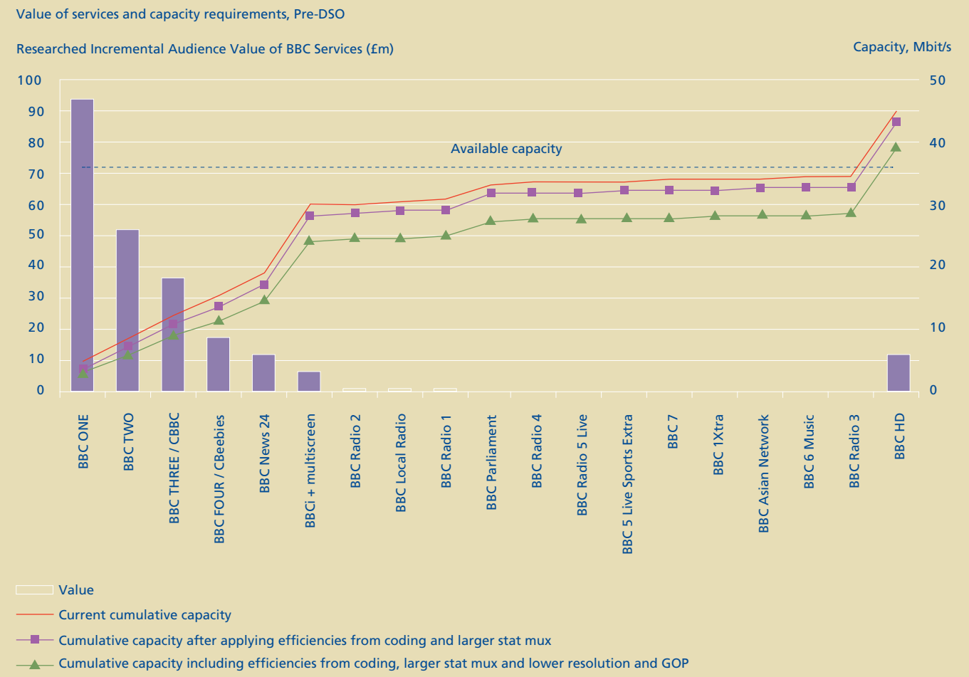
Figure 15 Incremental household value and use of available capacity by service, including efficiency gains, pre DSO
