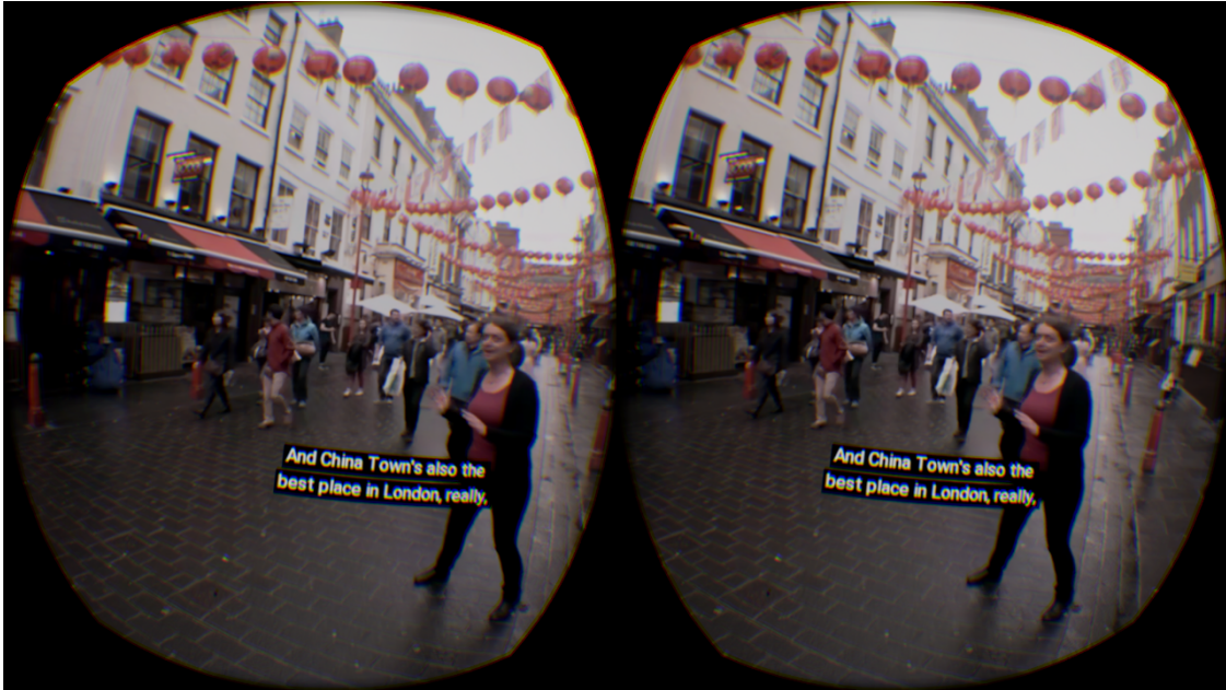
Figure 1: Screenshot from clip 1. The 360° video is projected onto the inside of a 25m diameter sphere, with the viewer at its center. The subtitles are displayed at 4m from the user with a visual style that aims to replicate that of standard subtitling on broadcast television, i.e., black background, fitted to text, sans-serif font.
