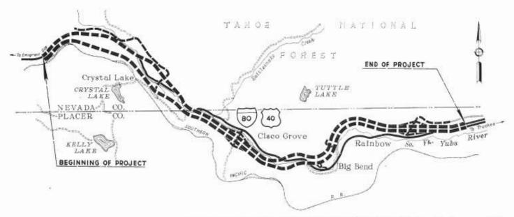
Heavy broken line shows general alignment of the SSR 20-Hampshire Rocks project. Narrow broken line shows access roads to recreational areas and interchanges. Solid line is existing highway, most of which will be preserved as frontage road. Frontage road and South Fork Yuba River run down median at two locations. Hampshire Rocks Campground is located near east end of project.
