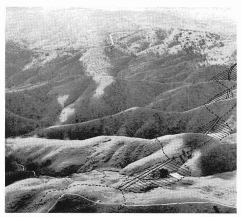
The proposed realignment drawn over this photo of the existing terrain shows location of the cut and fill portions. The present highway can be seen in the upper part of the photo.
