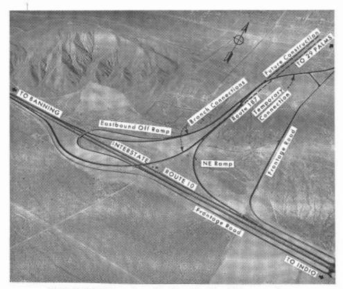
This aerial photo with superimposed text shows the design of the new interchange.
