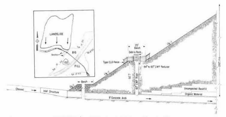
THE BIG FILL. The above sketch shows the arch culvert entrance and its secondary inlet.
