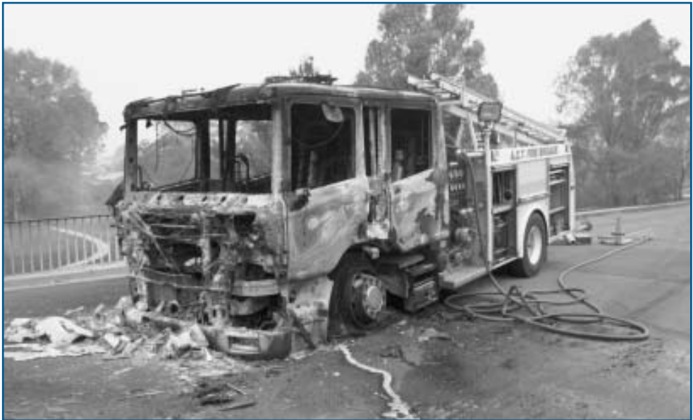
The ACT Fire Brigade pumper burnt due to embers entering the engine. Photo printed with permission of the Canberra Times .
