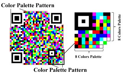
**Fig. 3.** The four *Color Palette Patterns* are pointed out in a HCC2D code using 8 colors. Figure taken from [17]. (Viewed better in color).
