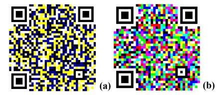
**Fig. 1.** Samples of the High Capacity Colored 2-Dimensional code (HCC2D): (a) 4 colors and (b) 8 colors. Figure taken from [17]. (Viewed better in color).
