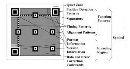
Fig. 2. Structure of generic QR codes and HCC2D codes, which inherit all function patterns of QR codes.
