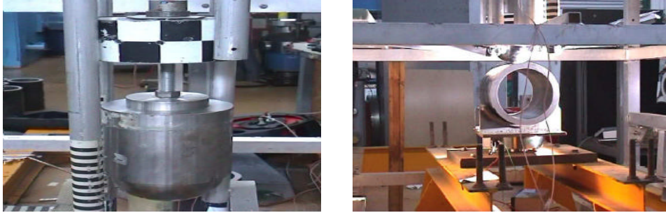
Figure 2. Instrumented drop weight set-up.
