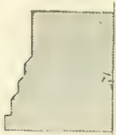
Section of Stone in foundation of side of Door
