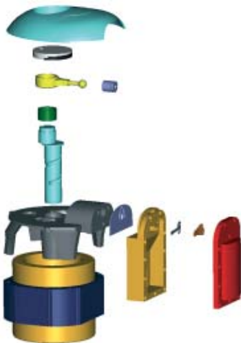
Schematic diagram of a hermetic compressor for CO 2 applications
