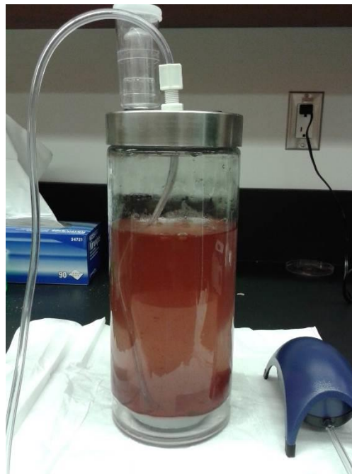
Figure 4.2: (b) The photobioreactor used for the study.
