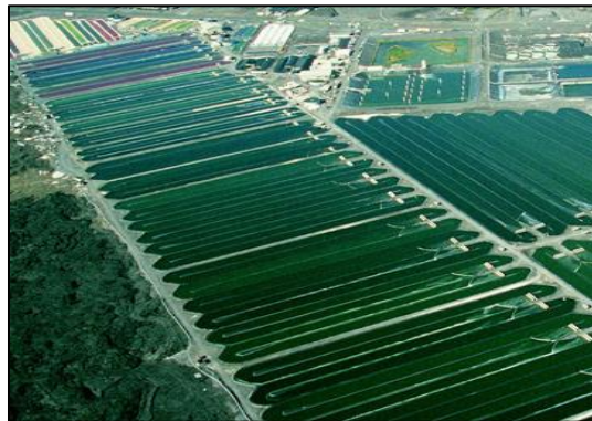
Figure 2.2: Paddle wheel Raceway pond used by Cyanotech Corporation, Hawaii.
