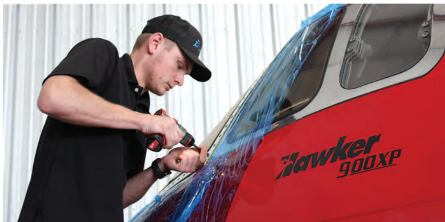
Plane Place co-owner and DOM Tristan Noe replacing a Hawker windshield.
