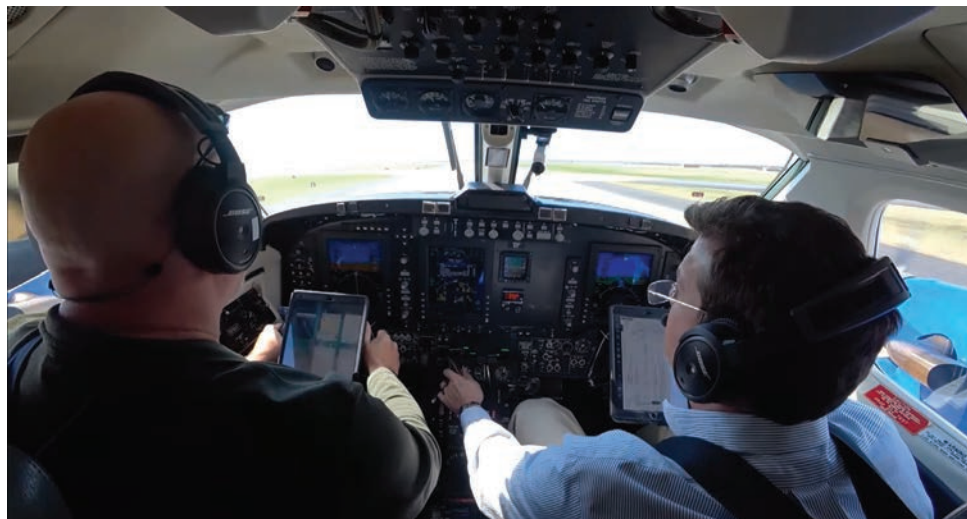
Flight inspection teams have to test every IFR procedure to ensure its safety.
