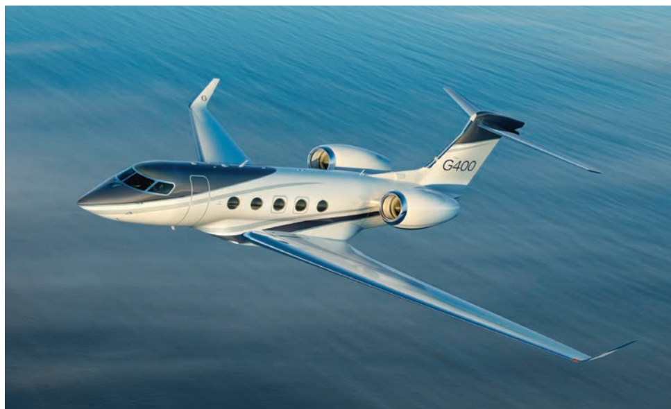
About 10 feet shorter than the G500, the G400 can fly 4,200 nm at Mach 0.85.
