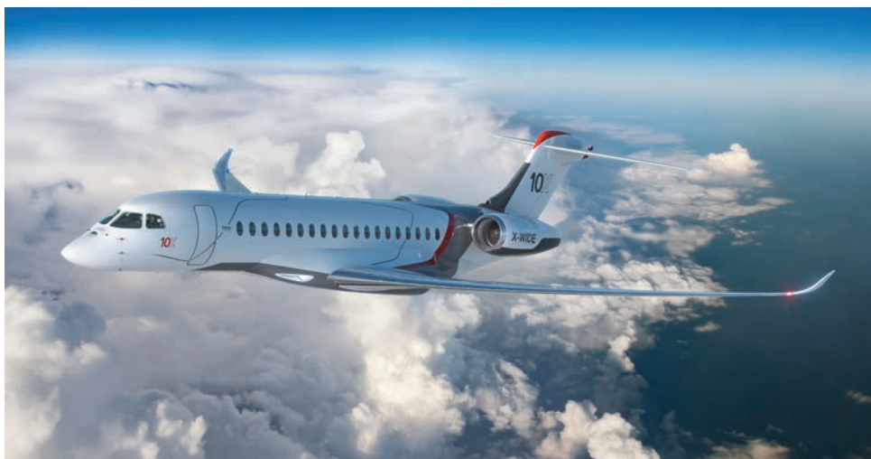
The 7,500-nm Falcon 10X will feature a unique single power lever and recovery mode.
