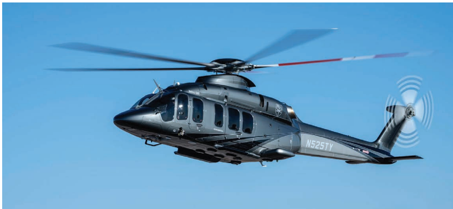
Bell's fly-by-wire 525 is the largest civil helicopter the company has ever built, designed to serve new medium twin markets.
