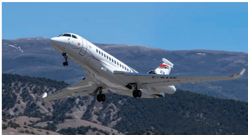
The $57 million Falcon 6X can take off with a balanced field length of 5,840 feet at mtow.
