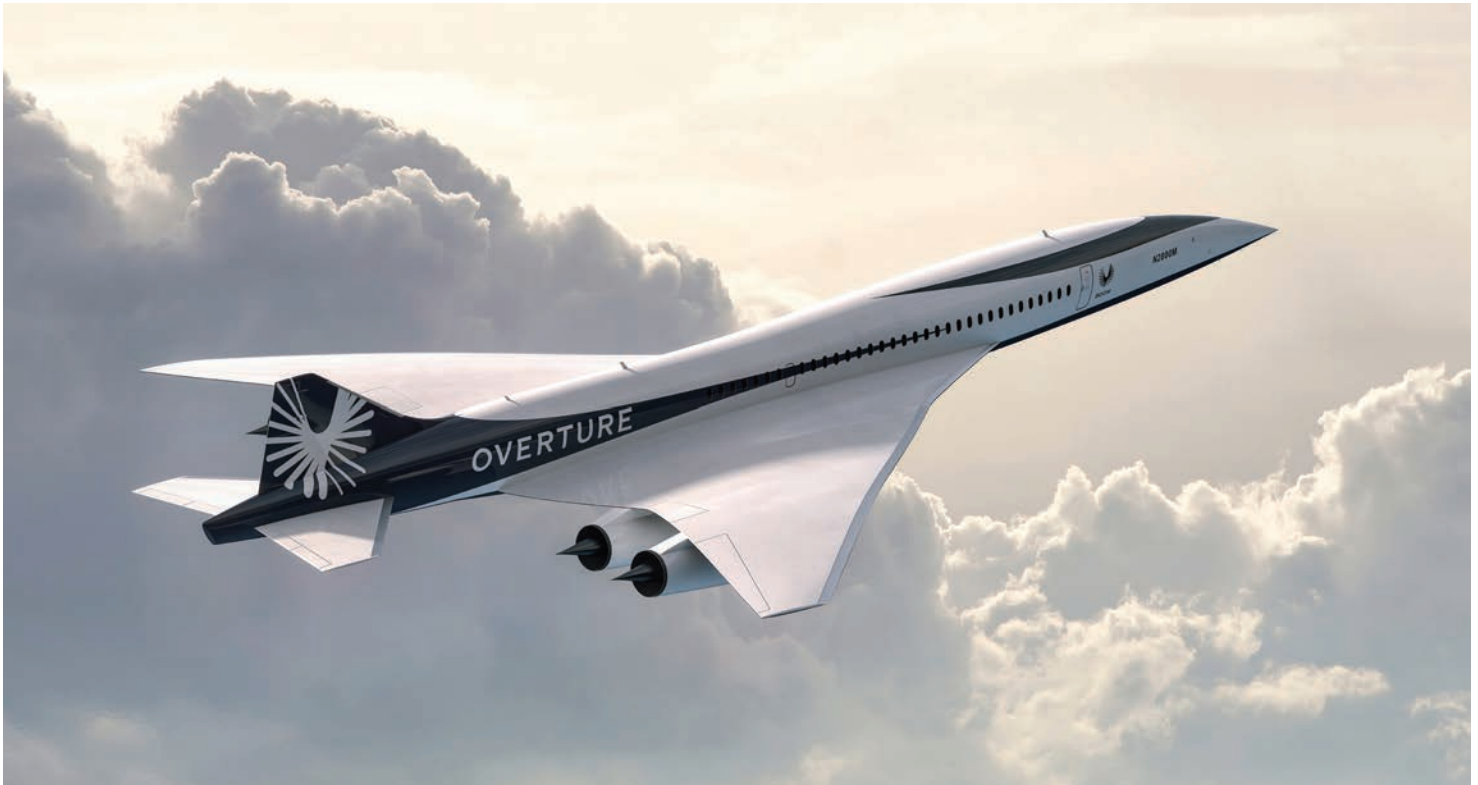
Boom's supersonic Overture will fly at maximum speed of Mach 1.7 and carry 65 to 80 passengers.
