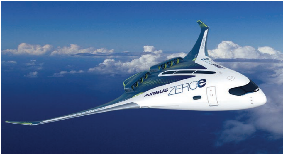
A blended-wing design is one of Airbus's Zero E conceptual aircraft configurations.
