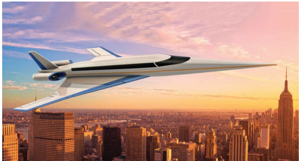
Spike Aerospace is targeting the business aviation market with the Mach 1.6 S-512 supersonic jet, which can carry up to 18 passengers while producing a “low boom” sonic boom.
