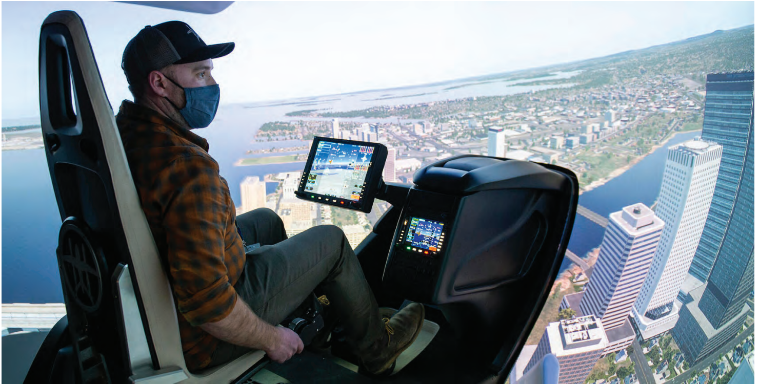
Simulating the simplified control system in the Beta Technologies Alia eVTOL aircraft.
