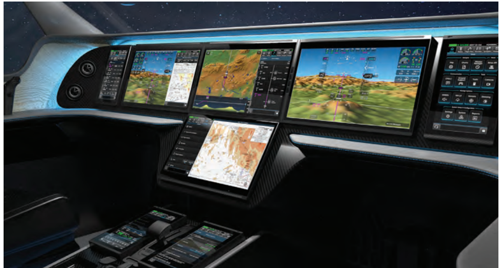
Honeywell’s Anthem avionics suite will incorporate voice command functions.
