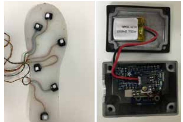
(Left) Prototype insole, showing multiple integrated pressure sensors. (Right) Prototype position sensor.
