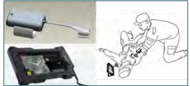
Ultrawide-Band, Wearable Ultrasound Probe for Battlefield Use
