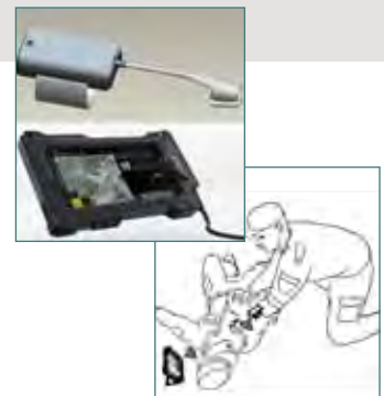
Ultrawide-Band, Wearable Ultrasound Probe for Battlefield Use
