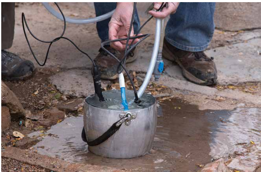
IAEA supports the many peaceful uses of nuclear energy. Pictured here is the use of a nuclear technique called isotope hydrology to study the quality of the local water supply in Mendoza, Argentina. In Argentina, as in many parts of the world, water is at risk of over-exploitation and contamination. To protect it, scientists are using nuclear technology to determine the quantity and quality of water supplies. They use naturally occurring isotopes as tracers and study water's isotopic composition to find out where groundwater comes from, how it travels, if it is recent or old, its recharge rate and whether it is polluted. IAEA supports countries through training, equipment and technical expertise in isotope hydrology.
