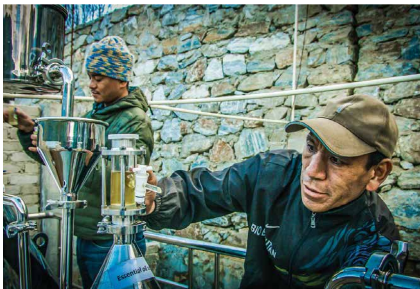
UNDP Bhutan has equipped a local private company, Bio-Bhutan, with a high-end steam distillation unit for the production of essential oils from rhododendron plants grown in the Dagala region of the country. Supported by UNDP, Bio-Bhutan is working with communities to develop natural products from rhododendron species in its Thimphu laboratories. 2017/UNDP BHUTAN - NPIF
